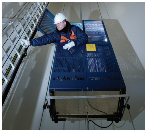
The Avanti Service Lift turns around its own axis and follows the ladder from the bottom to the top of the wind turbine.
